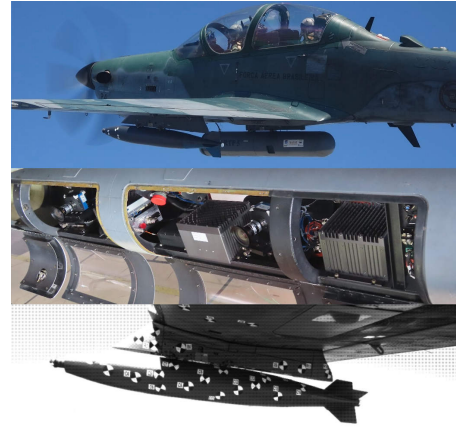
Fig. 1. A store separation flight test with an Embraer 314 (Super Tucano) conducting the test with a camera pod attached (middle) and its image captured before the separation (lower).
